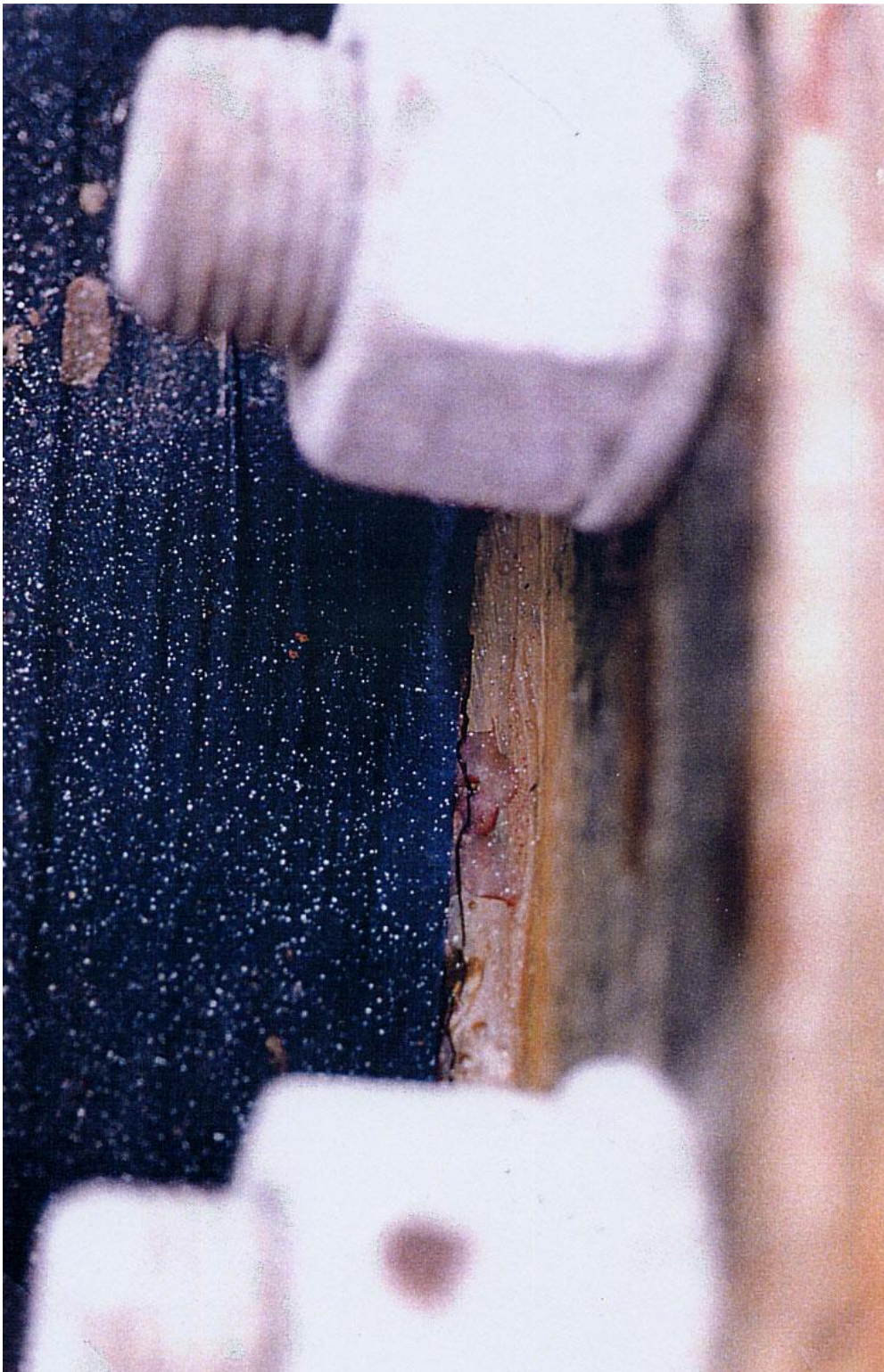
FIG. A17: Crack, in resin-rich surface layer. (A) View of flange (white particles are snow)
