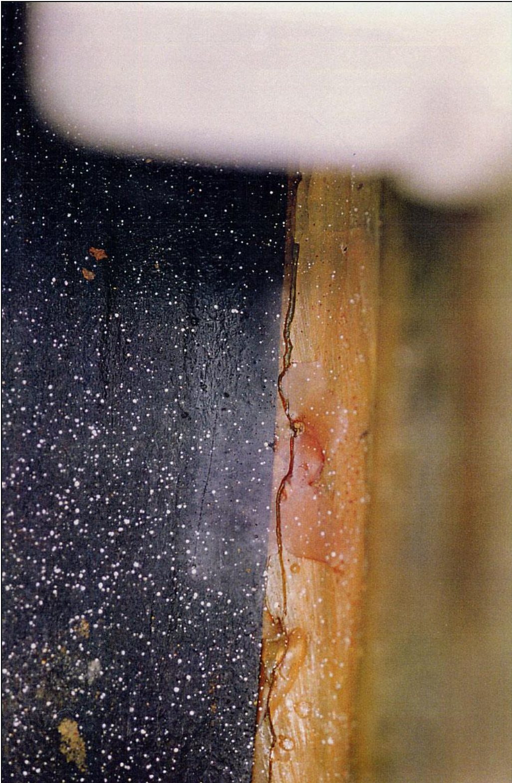
FIG. A17: Crack, in resin-rich surface layer. (B) Close-up view showing crack depth to surface resin layer thickness (white particles are snow)
