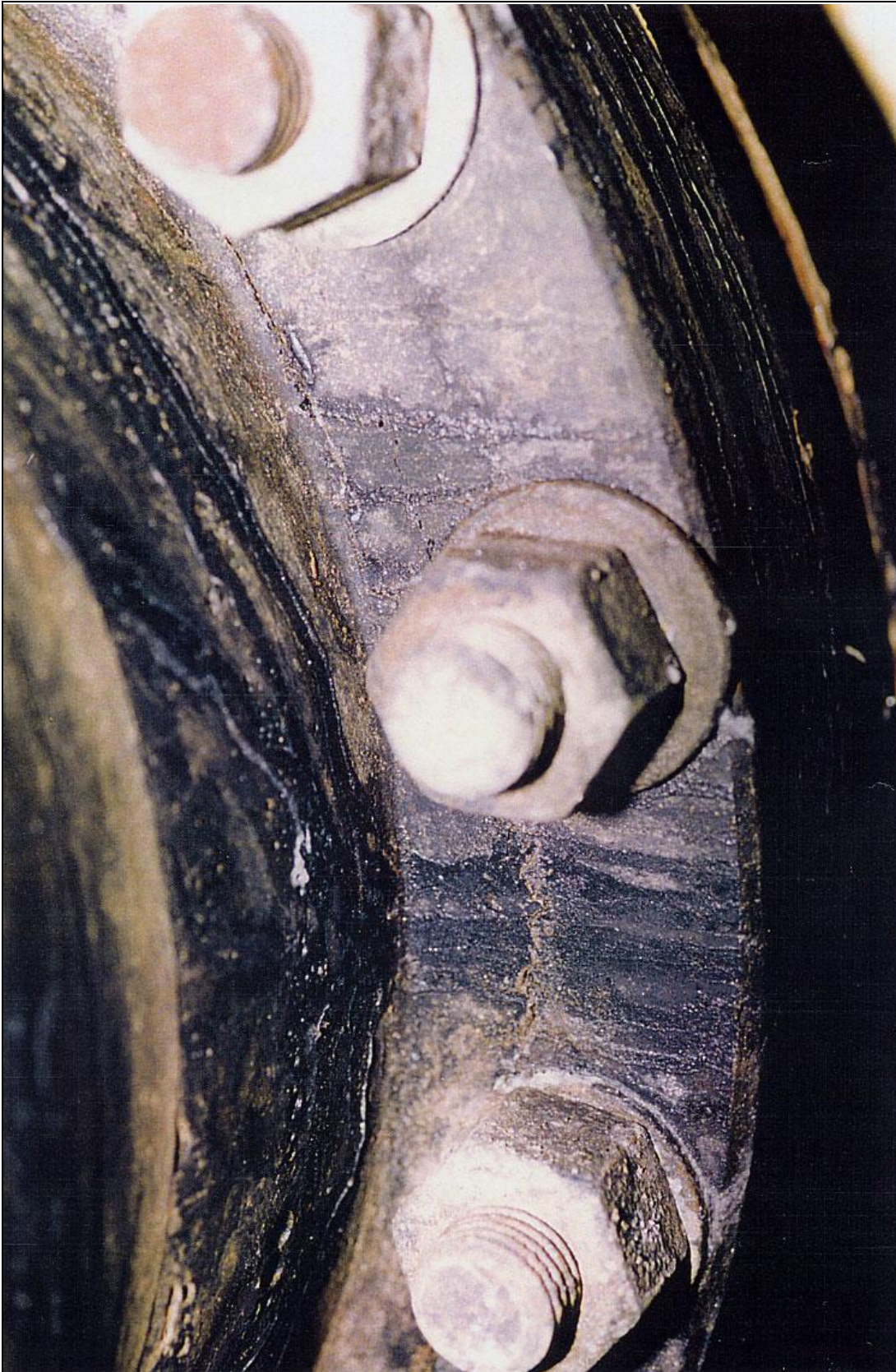
FIG. A16: Cracks, in flange root and bolt ring. Cracking caused by overtorquing bolts or overstressing flange (white on surface is salt)
