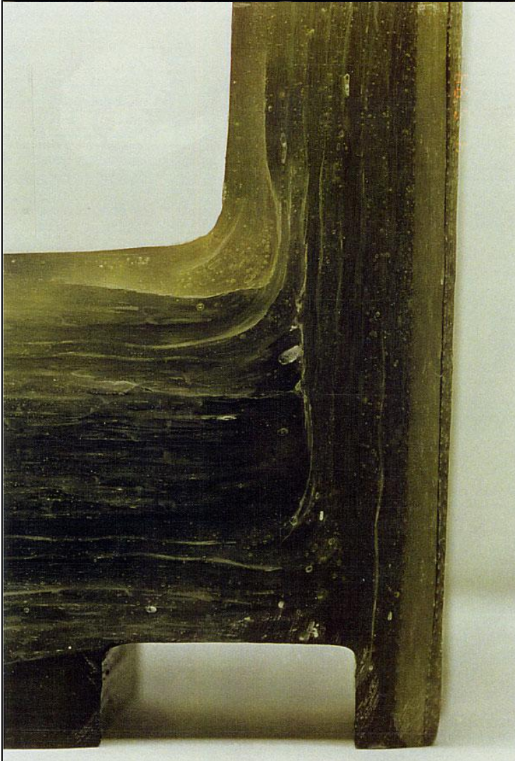
FIG. A10: Delamination. Internal. Delamination in flange root (caused by stressing flange with plies layed-up using incorrect sequence)
