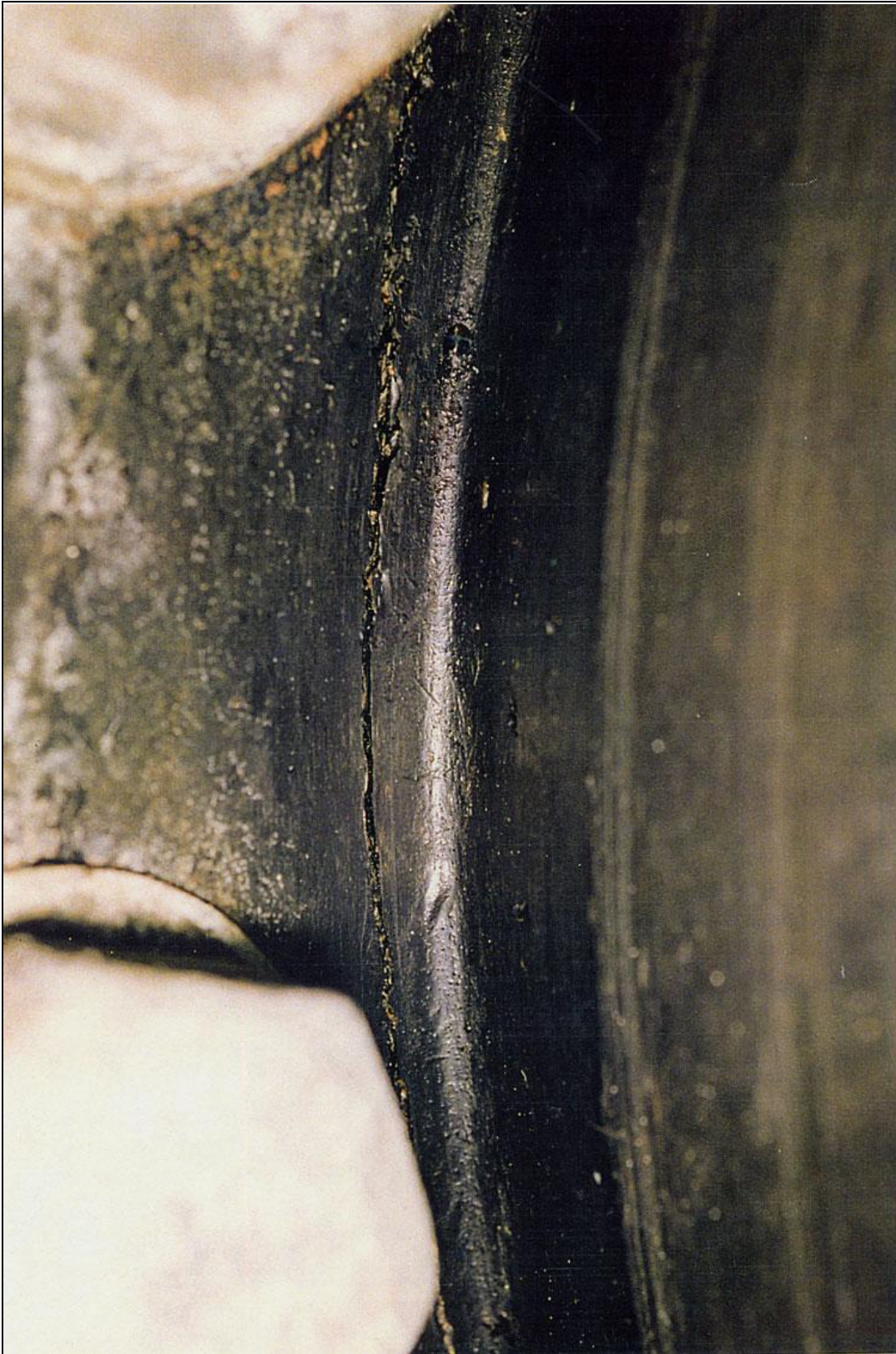
FIG. A15: Crack, in flange root. Detail showing typical cracking (not same flange as FIG. A14)
