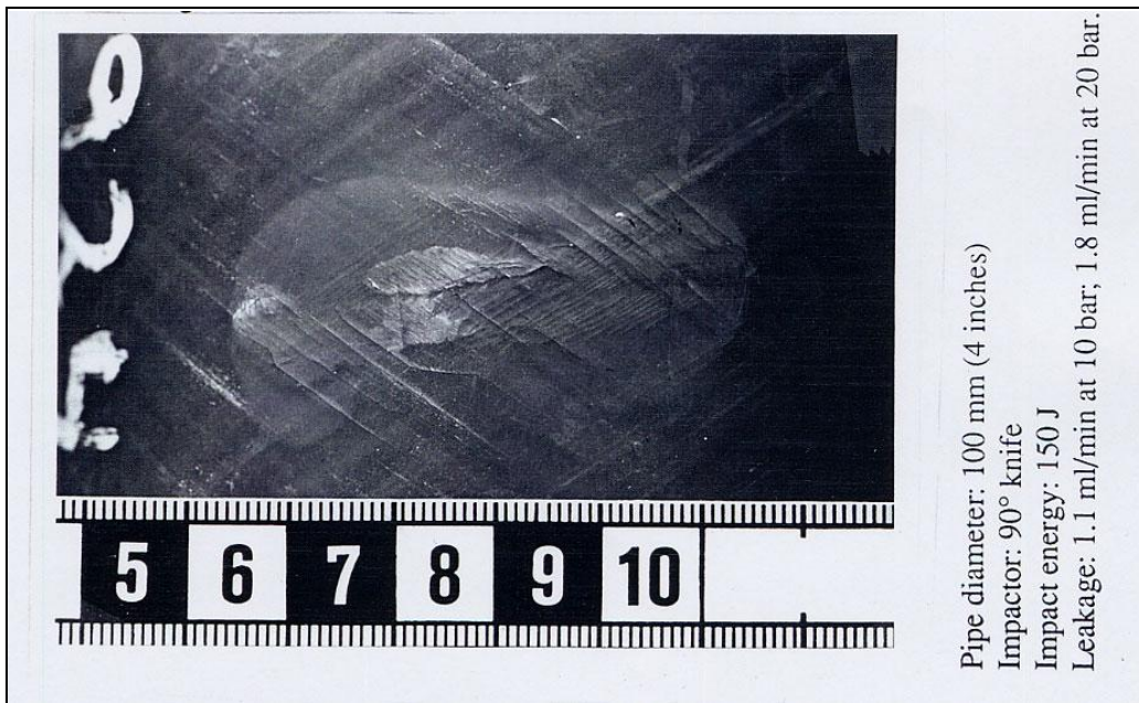
FIG. A8: Cracks. Delamination. Impact damage.
