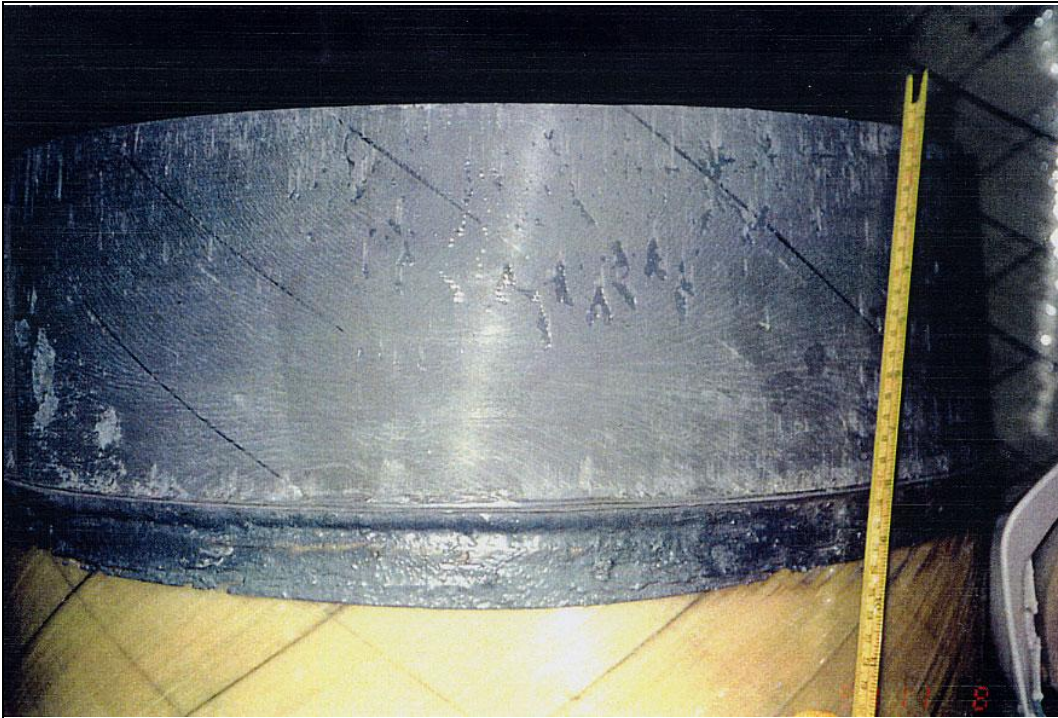
Taper spigot-end of 24" pipe
