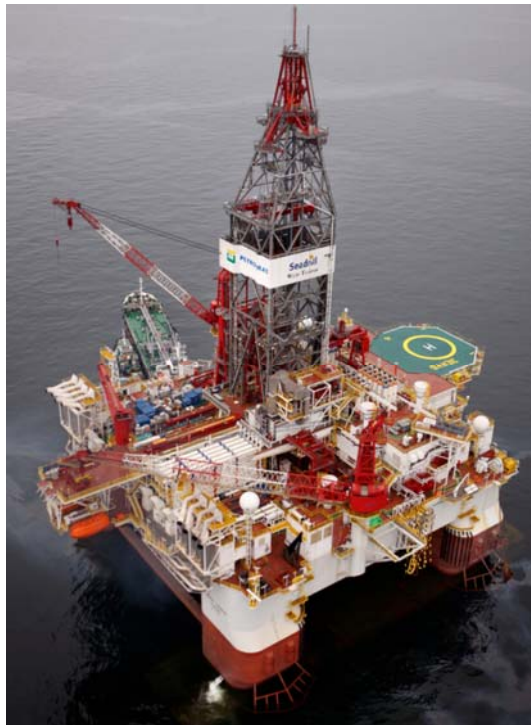
Figure 3-1: Semi-submersible drilling rig – Typically used in Norwegian waters
